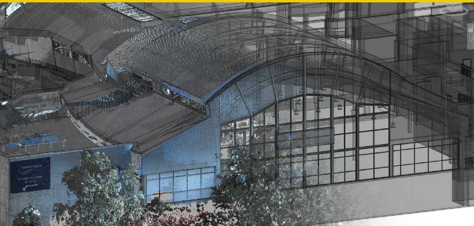
Image Blended image of a laser scan/point cloud survey (from left), transitioning to Revit model on right.
