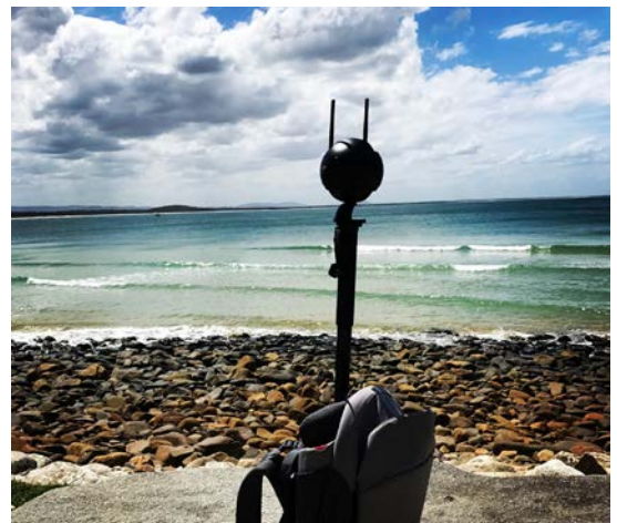
Image 3D spherical still and video camera for dilapidation reports, Google Street View updates, site tours, construction documentation
